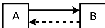
Figure 4.1: Using a weak reference to break the reference cycle between A and B.
